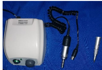
Figure (1) Micromotor & Handpiece
